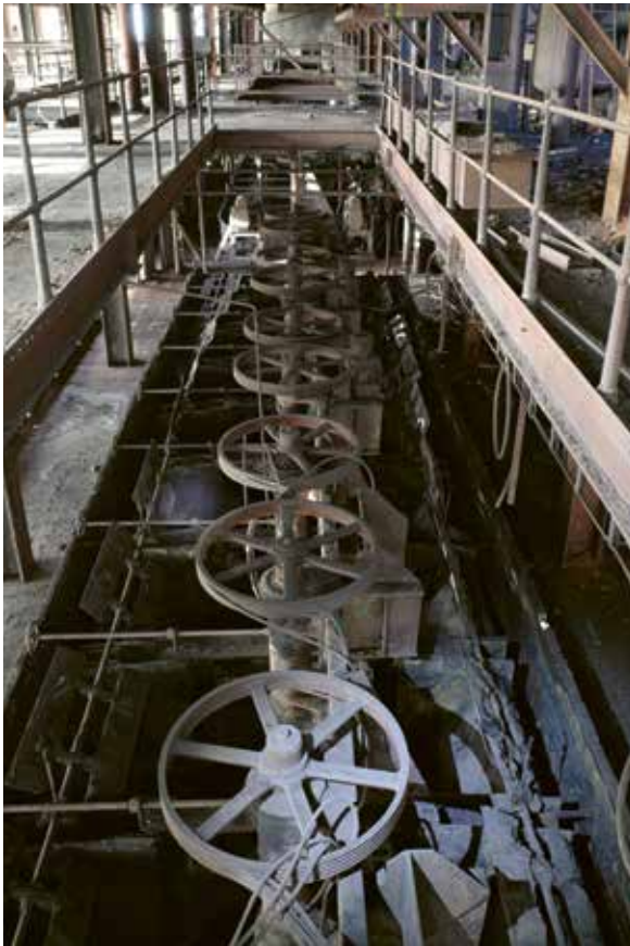
[photo above: slurry screen] [photo left: flotation battery] [photo bottom: flotation battery]
